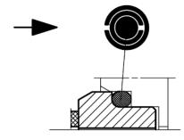
When using double-PTFE-wrapped o-rings care has to be taken that the joint on the outer wrapping faces against the assembly direction. Otherwise there is a risk of the wrapping opening and being pulled off, possibly resulting in seal leakage.
