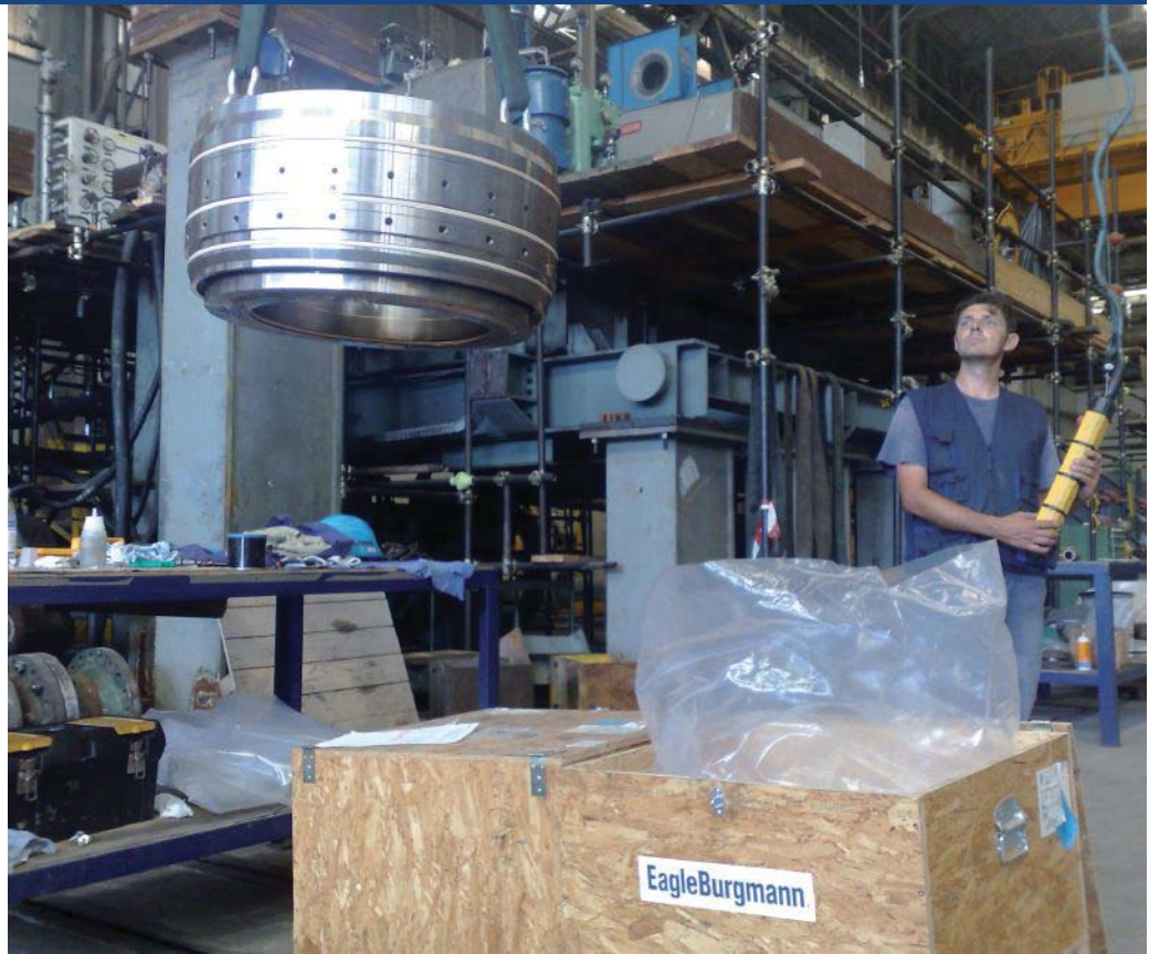
An EagleBurgmann 15.35 inch (390 millimeter) seal during preparation for shipment.
