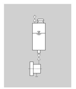
Install the quench fluid tank above the mechanical seal. Install connection pipes to the mechanical seal with low flow resistance. Pipes must vent automatically in the direction of the tank. It is imperative that air pockets are prevented.
